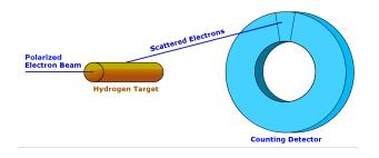
Beam :  $E_{\text{beam}} = 155 \, \text{MeV}$ ,  $I_{\text{beam}} = 150 \, \mu \text{A} = 10^{15} \, e^-/s$ ,
