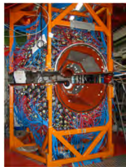
Figure : The Crystal-Ball is a 4\pi calorimeter around the main target [4]
